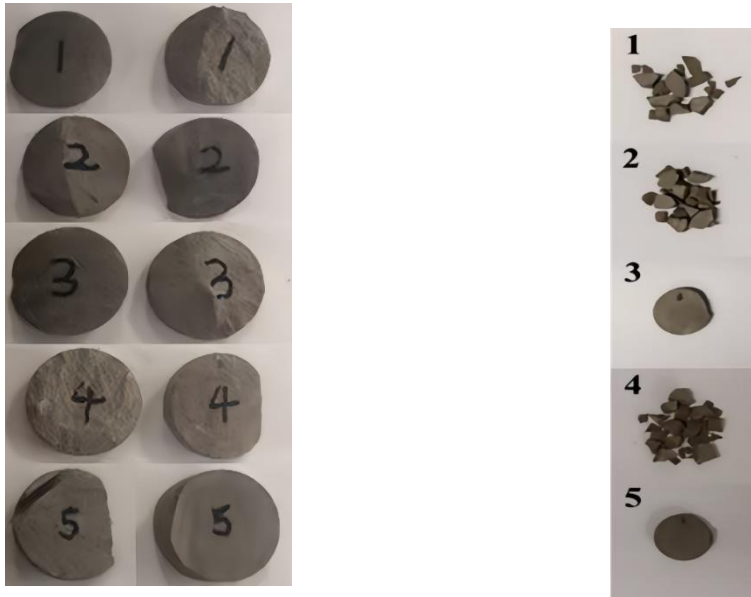
Fig. 2: Schematic diagram of the shale samples for X-ray diffraction.
